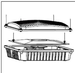
2. Cut off the wires through from 3/4" hole and plug the hole with provided Plug. Drill 4 holes on edge of fixture and fix it on the ceiling with using appropriate screws.
