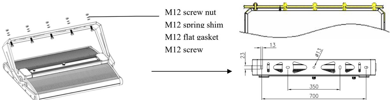
**Step 2:** Adjust the angle of the light bracket as per the illumination design and then tighten the screws
