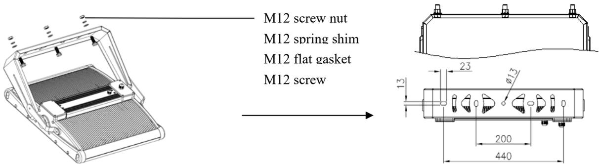
**Step 2:** Adjust the angle of the light bracket as per the illumination design and then tighten the screws
