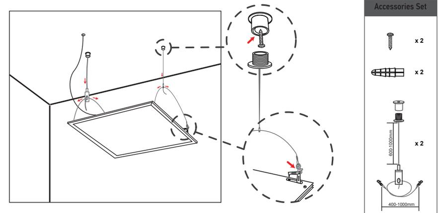
1. Make sure that the ceiling can hold the weight of the LED panel and install ceiling brackets suitable to support the weight of the LED panel. Fixing cables.
