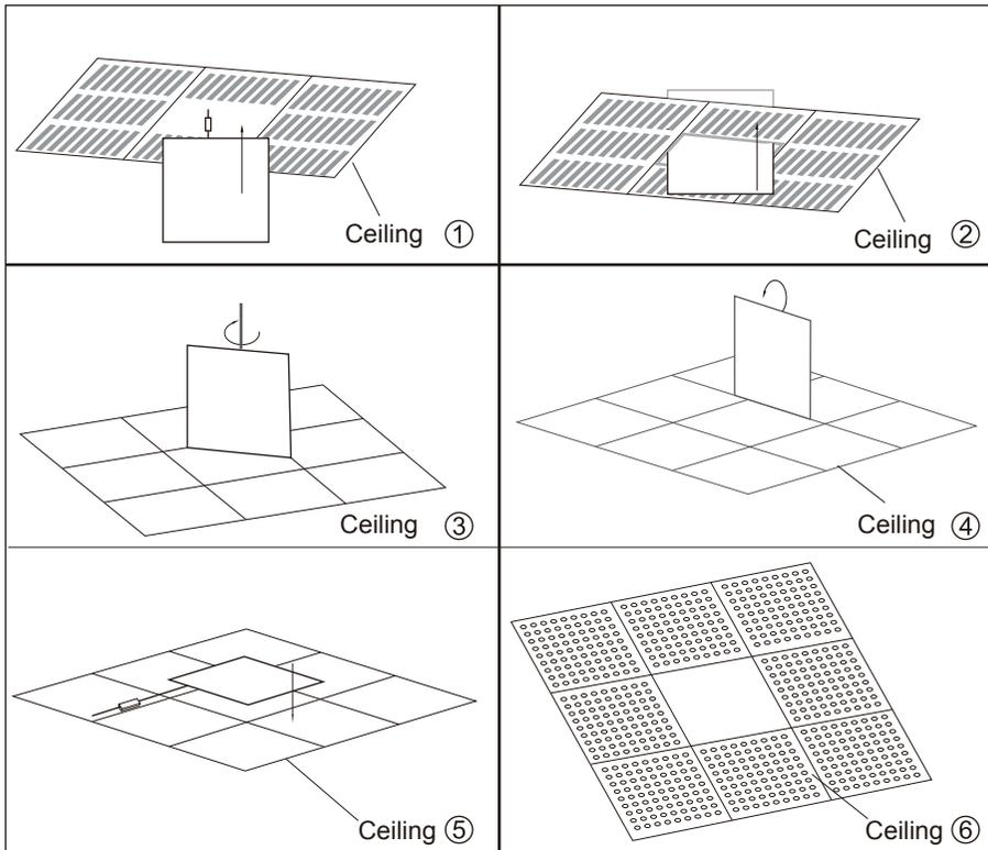
1. Ensure the panel light work well before installation, put the panel light at a diagonal position.
